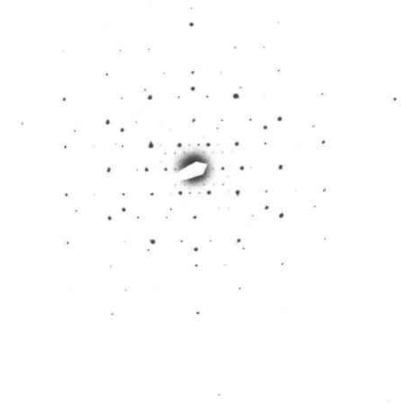
Fig. 7. Electron-diffraction pattern of the basal plane of gonyerite.
