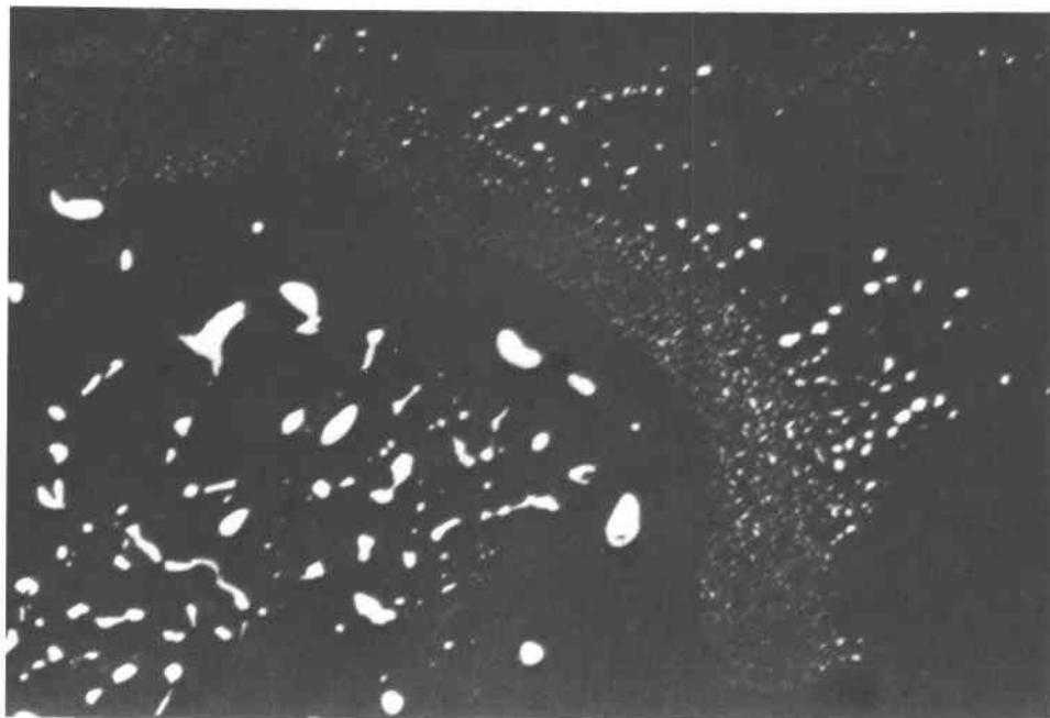
Fig. 1. Chalcopyrite (light) in a single crystal of sphalerite (dark), photographed in reflected light (oil immersion) showing varying sizes and irregular distribution of chalcopyrite blebs. Field width, 0.022 mm; specimen PBB (4) from Creede, Colorado.
