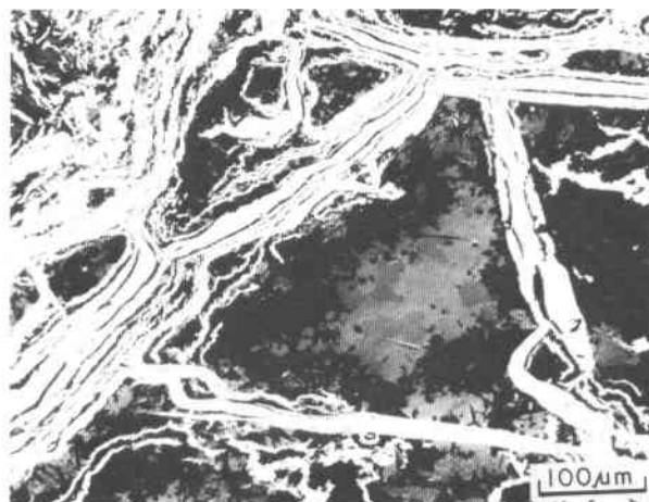
Fig. 2. Scanning-electron micrograph (back-scattered-electron image) of the same area as Fig. 1, but with the contrast between minerals greatly increased. Danielsite (light gray) and stromeyerite (slightly darker) occupy the center of the triangular area and are surrounded by chalcocite (black). The anglesite is white.
