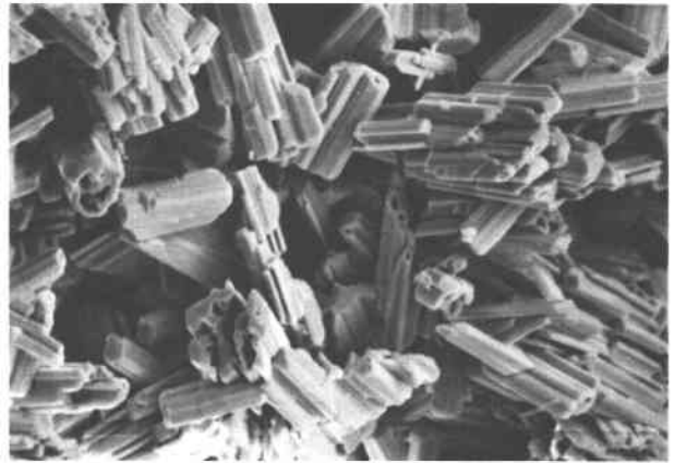
Fig. 2. SEM photomicrograph showing aggregates of perroudite crystals from Broken Hill, New South Wales. The crystals average about 0.025 mm long.
