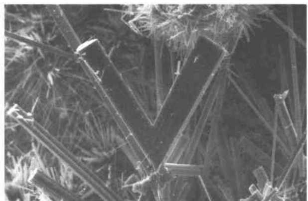
Fig. 3. SEM photomicrograph of a contact twin of perroudite from Cap-Garonne. Each arm of the twin is 0.08 mm long.
