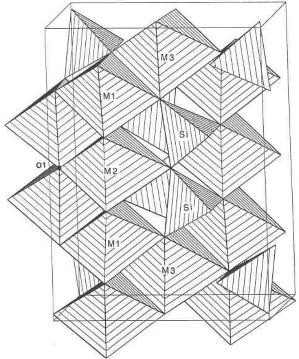
Fig. 1.  $\beta$ -Mg<sub>2</sub>SiO<sub>4</sub> structure, perspective *a*-axis projection, *c* horizontal. The Si<sub>2</sub>O<sub>7</sub> groups are clearly shown. This is a sorosilicate, not an orthosilicate or spinel. The O1 position (labeled) does not bond to Si and thus may be a potential site for water in the lower part of the upper mantle.
