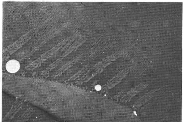
Fig. 6. Extensive growth of olivine from resorbed olivine interface, outward into the 77115 liquid in run slowly quenched from 1450°C (highly reflective phase is Fe°). Run 98; reflected light; width of field = 0.55 mm.
