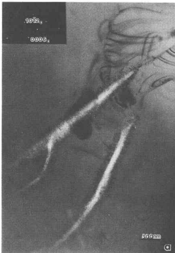
Fig. 2. (a) Incipient microfractures in aragonite due to rapid heating and transformation to calcite. (b) Microfractures separate as the thin foil shifts and buckles.
