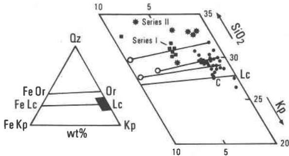
Fig. 4. Compositions of leucites in the West Kimberley lamproites (dots) compared with experimental leucite compositions in the system  $\text{SiO}_2\text{-KFe}^{3+}\text{SiO}_4\text{-KAlSiO}_4$  (after Carmichael, 1967). Squares = first series experiments; crosses = second series experiments; open circles = bulk scans of Al-spinel plus leucite host in West Kimberley lamproites.
