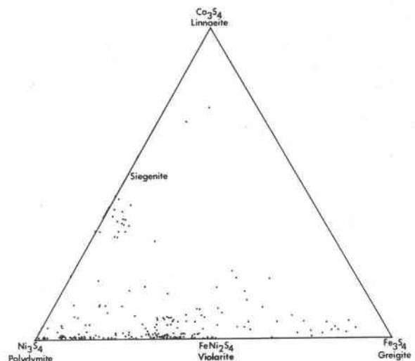
Fig. 7. Compositions of natural iron-nickel thiospinels shown in terms of  $\text{Fe}_3\text{S}_4$ – $\text{Ni}_3\text{S}_4$ – $\text{Co}_3\text{S}_4$  endmembers to illustrate the variation in cation contents (for sources of data see Table 2).
