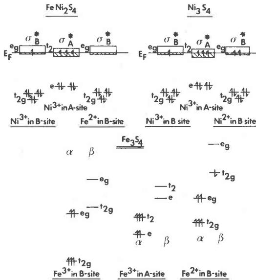
Fig. 9. Schematic energy level diagrams for the 3d orbitals in  $\text{Ni}_3\text{S}_4$ ,  $\text{FeNi}_2\text{S}_4$  and  $\text{Fe}_3\text{S}_4$ .  $\alpha$  and  $\beta$  refer to spin directions of the electrons;  $E_F$  is the Fermi level.
