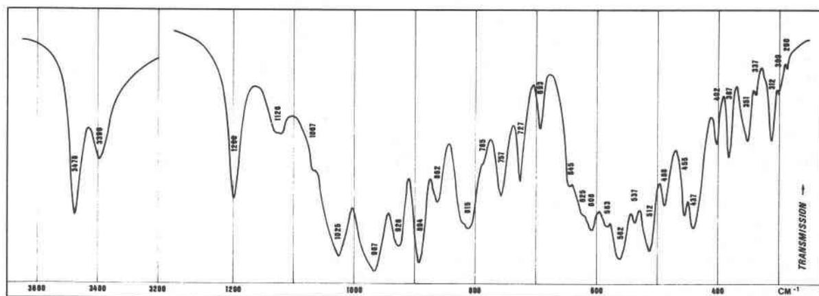
Fig. 1. Infrared spectrum of davreuxite from Ottré.
