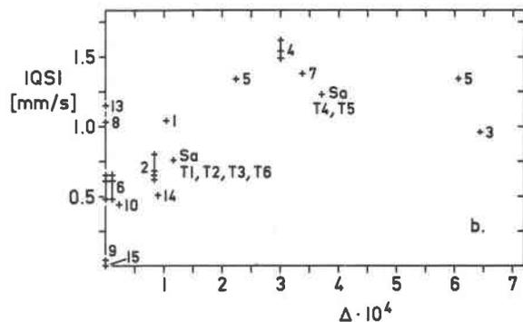
Fig. 4. Relationship between quadrupole splitting (QS) of tetrahedral ferric iron and the distortion parameters, bond angle variation  $\sigma^2$  (a) and bond length distortion  $\Delta$  (b), based on the data given in Table 5. Where more than one structurally distinct position may be suited for incorporation of ferric iron, their geometrical parameters have been plotted separately. The data for sapphire have also been plotted with the band assignment derived in the text (cf. Tables 2 and 4).
