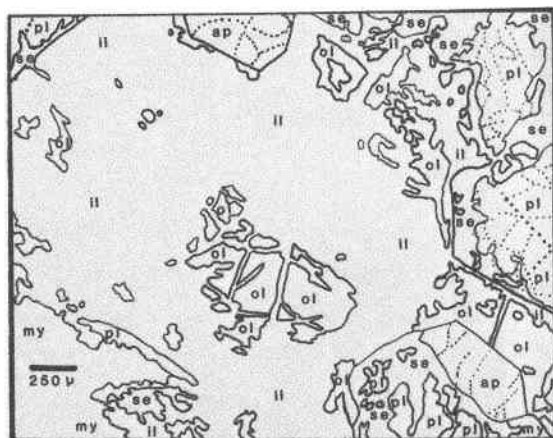
Fig. 1. Olivine grain in sample KG-247 75% replaced by ilvaite. Photo includes: grains of olivine (ol), ilvaite (il), plagioclase (pl), and apatite (ap); and patches of serpentine (se) and myrmekite (my).
