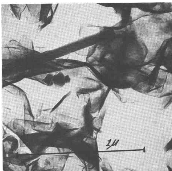
Fig. 4. Dimethyldioctadecyl ammonium smectite dispersed in benzene-methanol solutions and freeze-dried.
