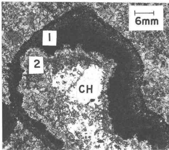
Fig. 5. Photomicrograph of chert nodule within dolostone showing a reaction rim of talc and calcite. The dark part of the reaction rim is growth within the dolomite matrix (1); the light part is growth with the chert (2). The clear part in the core of the nodule is chert (CH). Sample is 88 m from intrusive contact.
