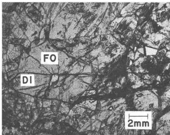
Fig. 10. Photomicrograph showing forsterite grain growing within diopside crystal. Note cracking of diopside crystal due to growth of forsterite. Sample is 567 m from intrusive contact.
