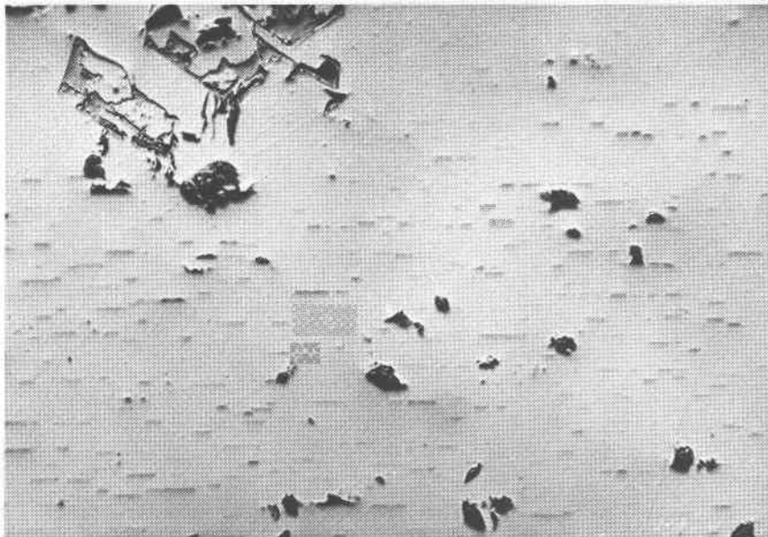
Fig. 8. Polished section of synthetic pyrrhotite formed by heating a synthetic iron-nickel sulphide melt in contact with a synthetic chromite and cooling over a period of 16 hours. Textures shown are of a grain boundary pyrrhotite/magnetite eutectic, and exsolution magnetite lamellae within the grains. Length of side 220\mu , crossed nicols.
