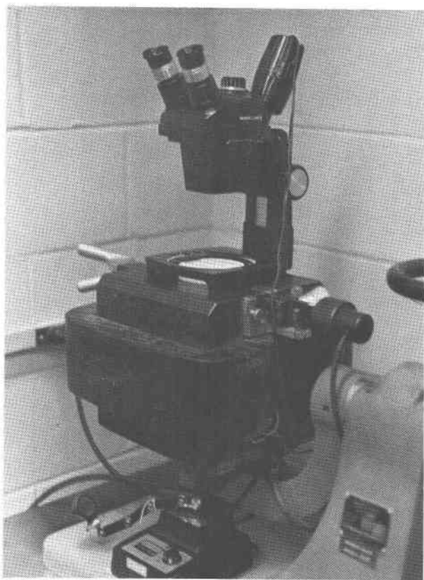
Fig. 2. Experimental configuration of microscope and Frantz Isodynamic Magnetic Separator used in magnetic-fluid method of density determination. Forward tilt of separator = 0^\circ , side tilt = 90^\circ .
