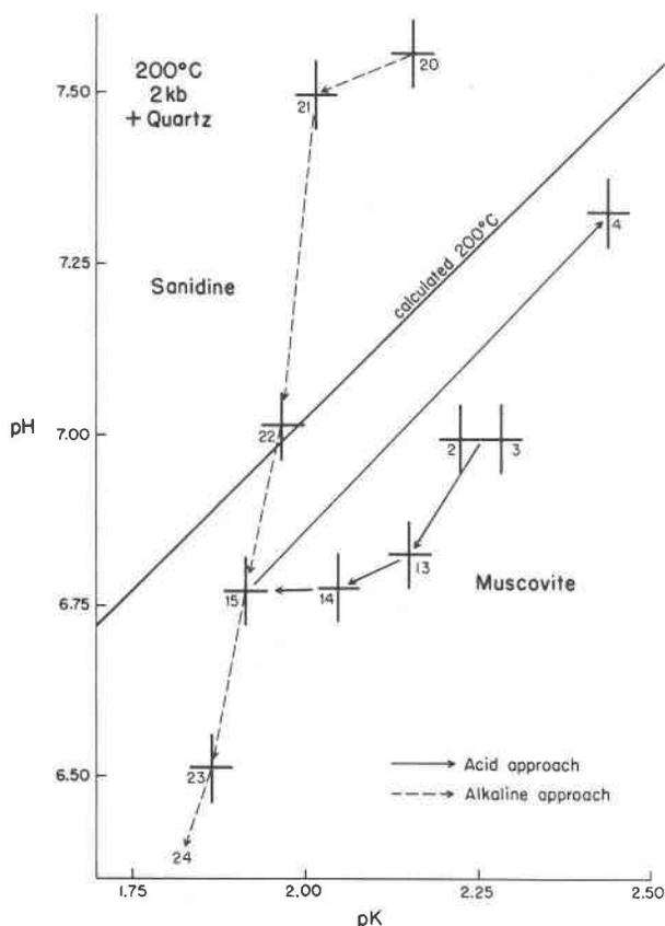
Fig. 5. Calculated ( $-\log a_{H^+}$ ) vs. calculated ( $-\log a_{K^+}$ ) for experiments conducted near  $200^\circ\text{C}$  at 2 kbar. The crosses indicate the uncertainties in the activities. The equilibrium constant calculated from thermodynamic data for minerals and aqueous species at  $200^\circ\text{C}$  is given by the slope of the solid line. See caption to Fig. 2 for more details.
