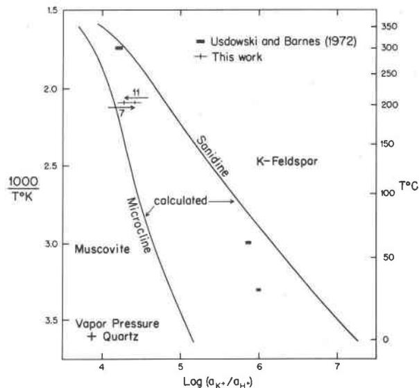
Fig. 6. The variation with temperature of the  $\log (a_{K^+}/a_{H^+})$  calculated from experiments of this study and from Usdowski and Barnes (1972). The equilibrium constants calculated theoretically for reaction 1 using alternatively microcline and sanidine are included for comparison.
