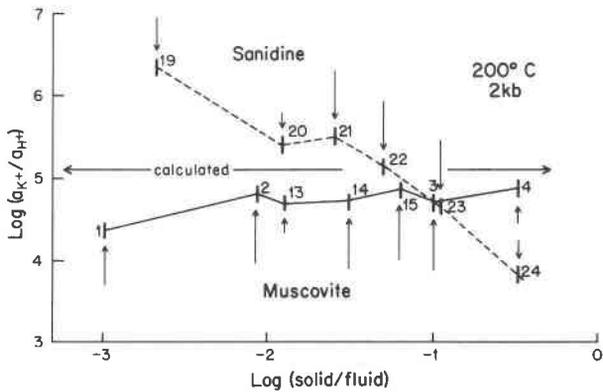
Fig. 3. Variation of  $\log(a_{K^+}/a_{H^+})$  vs.  $\log(\text{solid/fluid mass ratio})$  for reaction 1 at 200°C and 2 kbar total pressure. The horizontal line indicates the equilibrium constant for reaction 1 calculated from thermodynamic data—see caption to Fig. 2 for more details.
