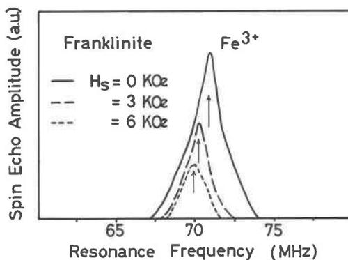
Fig. 7. External magnetic field dependence of  $^{57}\text{Fe}$  NMR of  $\text{Fe}^{3+}$  ions in franklinite at 1.6 K. Decreasing resonance frequency means that hyperfine field of  $\text{Fe}^{3+}$  ion in franklinite is antiparallel to external magnetic field.
