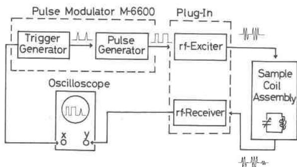
Fig. 1. Block diagram for pulsed NMR experiment.
