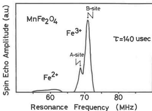
Fig. 5. Spin-echo spectrum of  $^{57}\text{Fe}$  NMR of powdered manganese ferrite  $\text{MnFe}_2\text{O}_4$  specimen at 1.6 K under zero external magnetic field. Double peak corresponds to  $^{57}\text{Fe}$  NMR of  $\text{Fe}^{3+}$  ions at A and B sites as indicated. Weak spectrum around 60 MHz is due to  $^{57}\text{Fe}$  NMR of  $\text{Fe}^{2+}$  ions at B sites.
