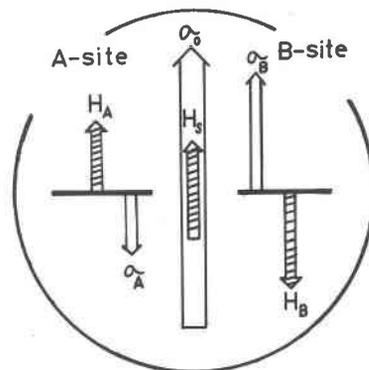
Fig. 8. Mutual direction between each sublattice moment ( $\sigma_A$ ,  $\sigma_B$ ) and each hyperfine field ( $H_A$ ,  $H_B$ ) in ferrimagnetic spinel under application of saturating external magnetic field ( $H_s$ ) when B-sublattice moment dominates. Resultant moment ( $\sigma_0$ ) is parallel to external magnetic field.
