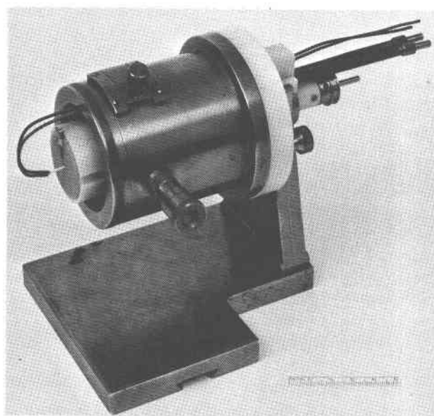
Fig. 1. The assembled low-temperature powder camera with film cassette in position (photograph by John Hall).
