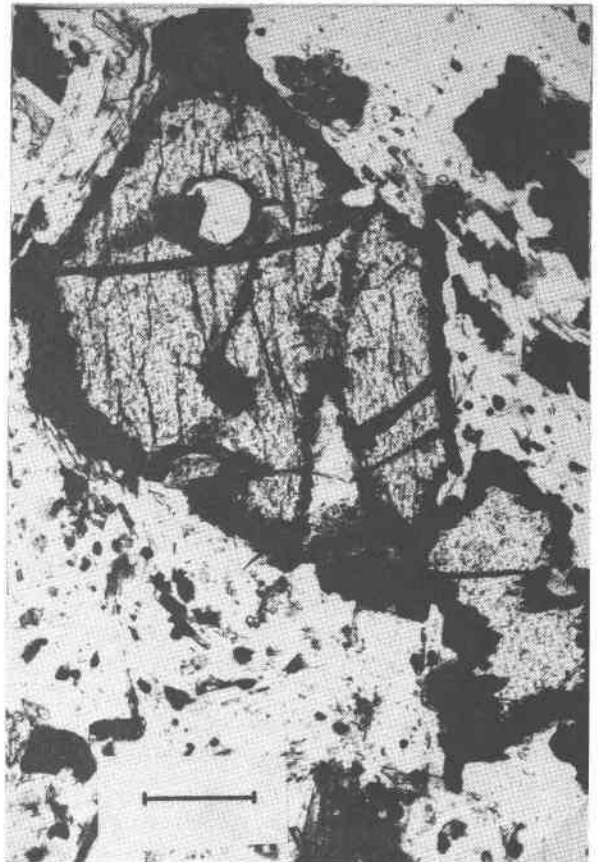
Fig. 2. Olivine crystal, rimmed by iron oxides. Length of the bar is 0.10mm.
