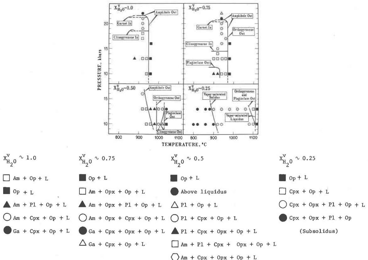
Fig. 1. Crystallization sequence for Mt. Hood andesite at  $X^V H_2O \sim 1.0, 0.75, 0.5$ , and  $0.25$ . All assemblages coexist with vapor. Abbreviations: Am—amphibole; Cpx—clinopyroxene; Ga—garnet; L—glass interpreted to be quenched liquid; M—micaceous mineral; Ol—olivine; Op—opaque mineral; Opx—orthopyroxene; Pl—plagioclase; q—interpreted to have crystallized during the quench; ?—questionable; ( )—trace amount.
