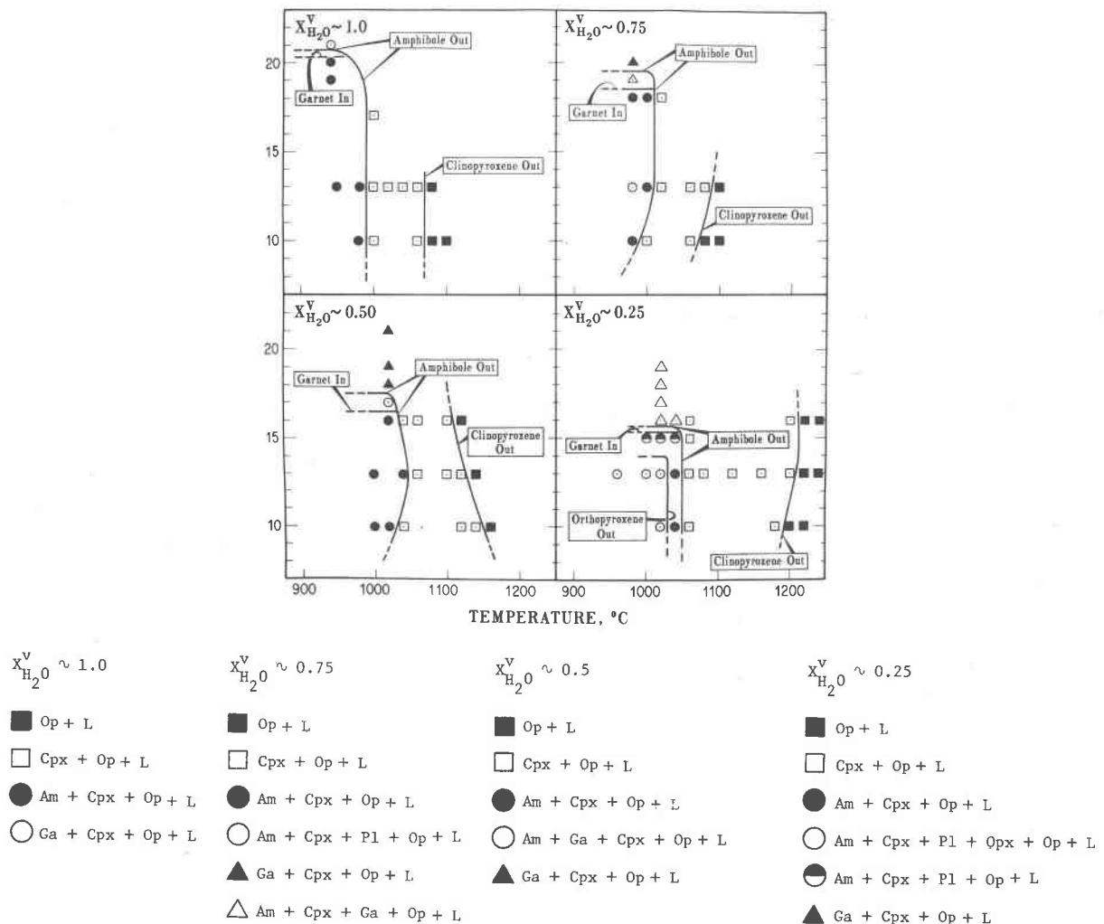
Fig. 2. Crystallization sequence for 1921 Kilauea olivine tholeiite at  $X^V_{H_2O} \sim 1.0, 0.75, 0.5$ , and  $0.25$ . All assemblages coexist with vapor. Trace amounts of olivine occur in some runs (see Table 1). See Fig. 1 for abbreviations.
