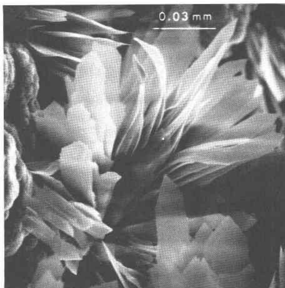
FIG. 4. Scanning electron micrography, showing individual crystals of cowlesite from Spray, Oregon. Compare the crystal in lower right corner with Figure 5a.
