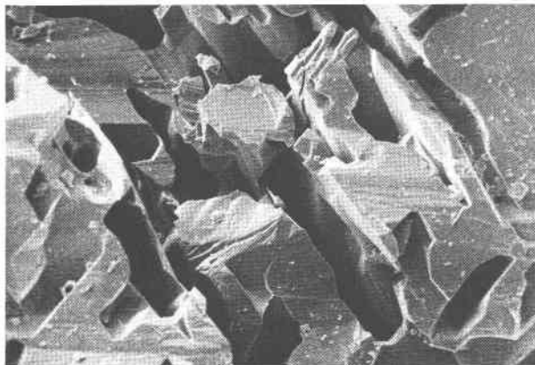
FIG. 5. SEM photo (500 \times ). Section of the translucent region in the 1.53 ct. Arkansas diamond. Relatively large flattened cavities were common to the 2.06 and 1.53 ct. diamonds (see Fig. 2), but more abundant in the latter. Long edge of photo = 200 \mu m.
