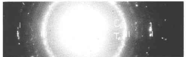
FIG. 8. Diffraction pattern from initially amorphous opal from Andamooka (S1) after being heated to 1200^{\circ}\text{C} for 3 hours. This diffraction pattern comes from an area containing many fragments.
