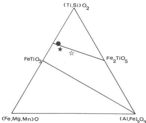
FIG. 3. Composition of Smoky Butte ferric armalcolite (solid star) compared to a lunar armalcolite (solid circle) analysis from Haggerty *et al.* (1970) and to a Hawaiian ferropseudobrookite (open star) analysis (FPSB 13 in Anderson and Wright, 1972).
