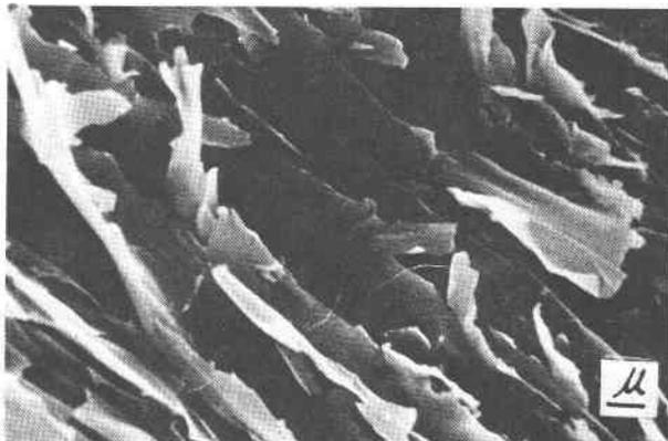
FIG. 4. Scanning electron photomicrograph of swinefordite.
