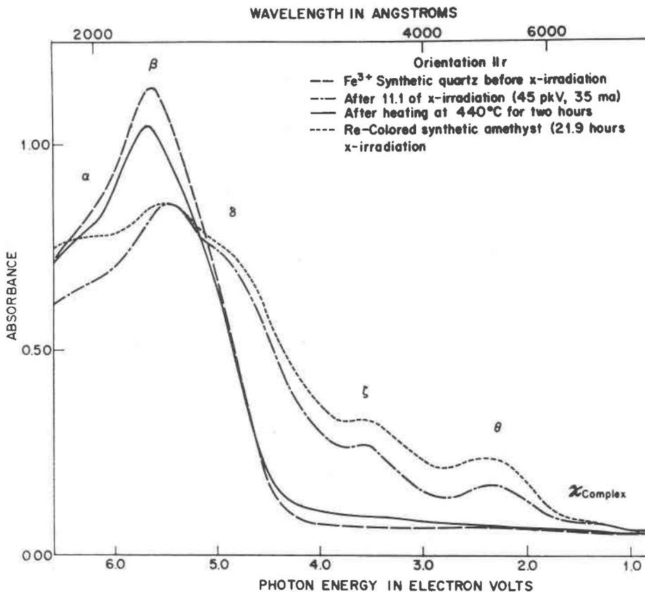
FIG. 8. Absorption spectra for normal incidence of light on a section of synthetic Fe<sup>3+</sup>-doped  $\alpha$ -quartz (H-95) cut parallel to positive rhombohedral face before and after X irradiation, after thermal bleaching and after recoloration.
