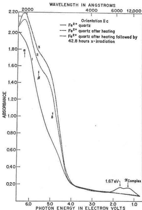
FIG. 11. Absorption spectra for normal incidence of light on a section of Fe<sup>2+</sup> quartz (A-84) cut parallel to the c axis after heating at 500°C for three hours, and after heating followed by 42.8 hours of X irradiation.
