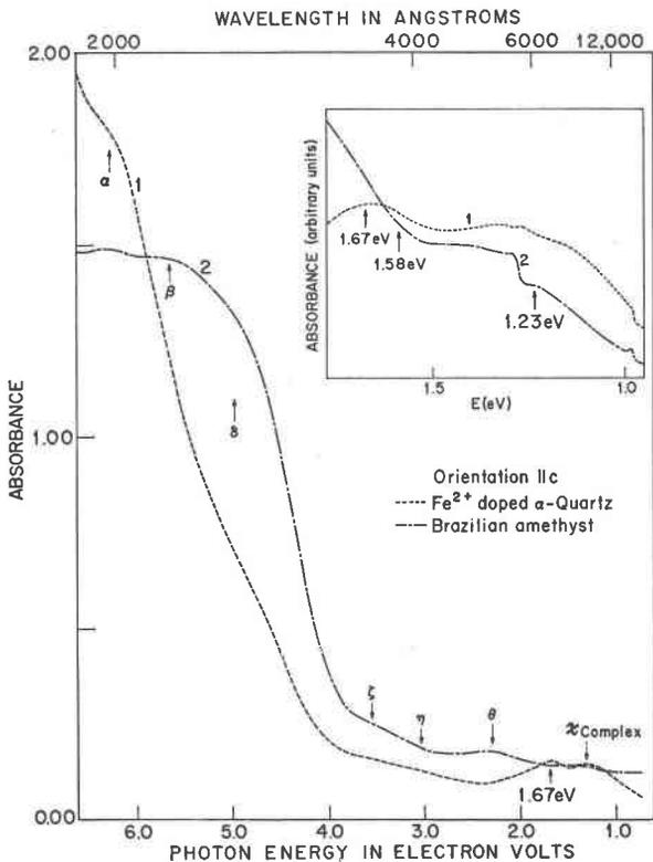
FIG. 1. Absorption spectrum for normal incidence of light on a section cut parallel to the  $c$  axis of synthetic  $\alpha$ -quartz (A-84) doped with trace Fe<sup>2+</sup> ion.
