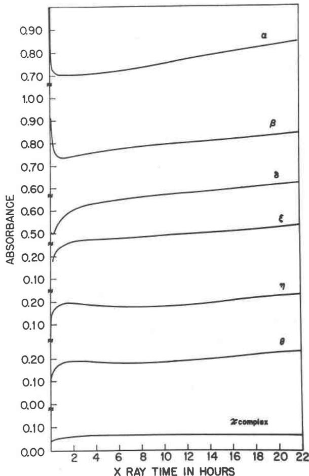
FIG. 6. The growth characteristics of the bands observed in a synthetic Fe<sup>3+</sup>-doped  $\alpha$ -quartz (H-95) section cut parallel to a positive rhombohedral face upon X irradiation.
