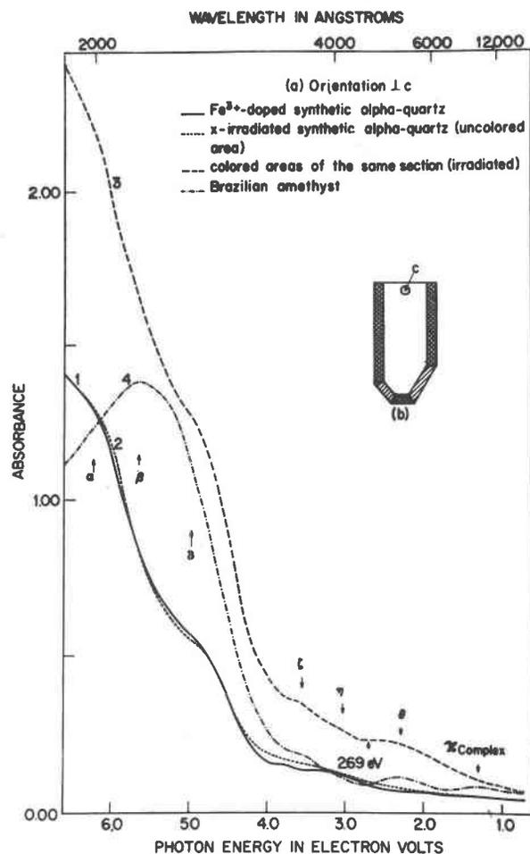
FIG. 5. (a) Absorption spectra for normal incidence of light on a section cut perpendicular to the  $c$  axis of  $\text{Fe}^{3+}$ -doped synthetic  $\alpha$ -quartz (Y-5) before and after X irradiation; (b) the section investigated (inset).
