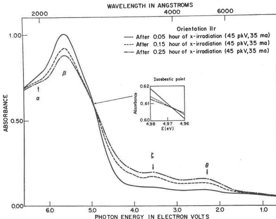
FIG. 7. Variation of the absorption spectrum with time of X irradiation of a section cut parallel to a positive rhombohedral face of synthetic  $\alpha$ -quartz (H-95), doped with  $\text{Fe}^{3+}$  ions.
