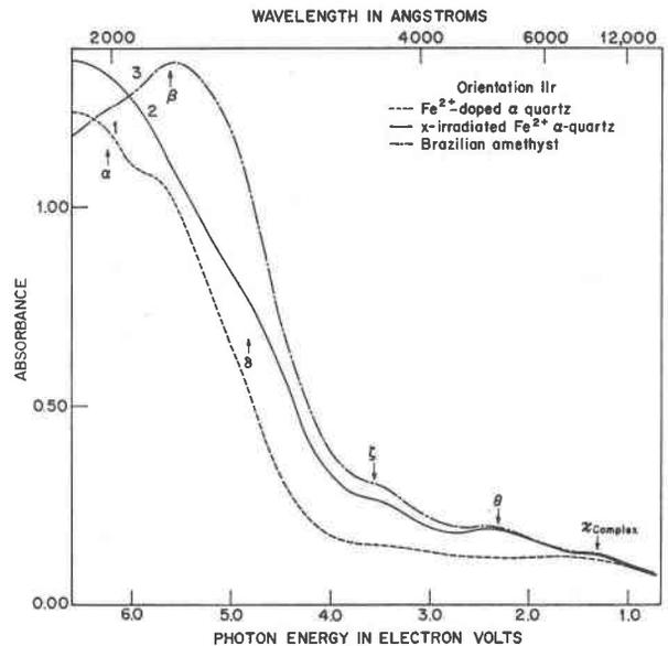
FIG. 3. Absorption spectra for normal incidence of light on a section cut parallel to a positive rhombohedral face of synthetic  $\alpha$ -quartz (A-84) doped with trace Fe<sup>2+</sup> ion before and after X irradiation.
