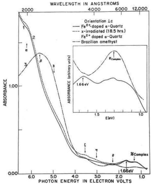
FIG. 2. Absorption spectra for normal incidence of light on a section cut perpendicular to the  $c$  axis of synthetic  $\alpha$ -quartz (A-84) doped with trace Fe<sup>2+</sup> ion before and after X irradiation.
