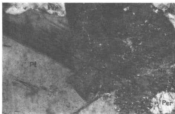
FIG. 3. Plagioclase and 'patch' nepheline relationship. Nepheline (Ne) boundaries show diffuse borders (d) along the contact of plagioclase (Pl). The indistinct cleavage and cracks in nepheline (Ne) are parallel to the twinning in plagioclase (marked by a line). The perthite blebs in nepheline are optically continuous with the outside perthite grains (crossed nicols, \times 40 ).
