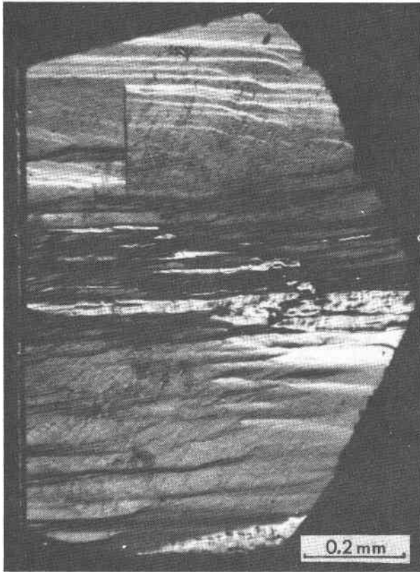
FIG. 5. Interference contrast photomicrograph of (210) face of a larger size crystal from the Shakanai mine, showing growth layers elongated parallel to the negative striations.
