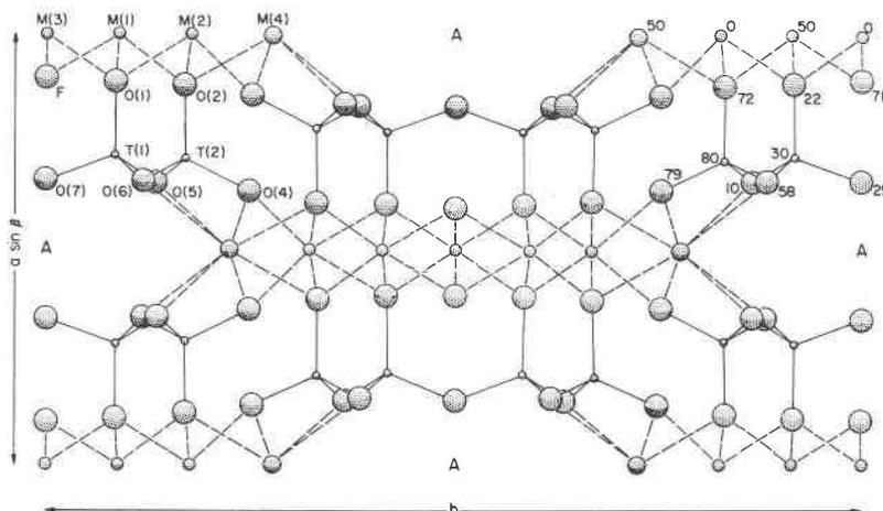
FIG. 1. The structure of tremolite projected down  $c$ . The nomenclature of the atoms is given in the upper left corner and the  $z$  fractional coordinates in the upper right. The vacant  $A$  site is indicated in this figure by the letter  $A$ .
