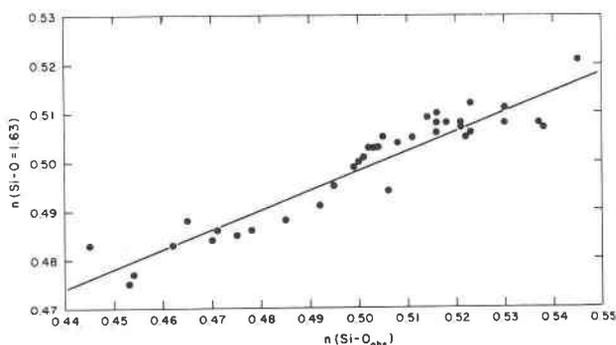
FIG. 2. Variation of  $n(\text{Si-O} = 1.63)$  with  $n(\text{Si-O}_{\text{obs}})$  for nine silicates using data from Gibbs *et al* (1971). [ $n(\text{Si-O} = 1.63)$  is calculated using constant bond lengths of  $1.63\text{\AA}$  and  $n(\text{Si-O}_{\text{obs}})$  is calculated using observed bond lengths.] The  $n(\text{Si-O})$  values were calculated assuming constant  $\text{Si-O}$  bond lengths, observed  $\text{O-Si-O}$  angles, and  $s$ - and  $p$ -basis functions.
