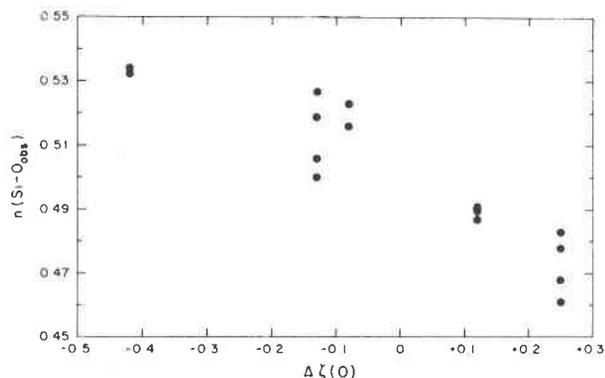
FIG. 3. Variation of  $n(\text{Si}-\text{O}_{\text{obs}})$  with  $\Delta\zeta(\text{O})$  for hydroxyl and fluor-tremolite.  $\Delta\zeta(\text{O}) = \zeta(\text{O}) - \langle\zeta(\text{O})\rangle$  where  $\zeta(\text{O})$  is the sum of Pauling bond strengths received by oxygen and  $\langle\zeta(\text{O})\rangle$  is the mean  $\zeta(\text{O})$  in a given tetrahedron.
