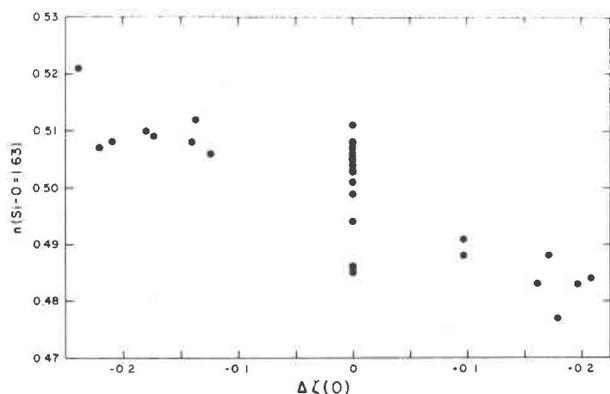
FIG. 4. Variation of  $n(\text{Si}-\text{O} = 1.63)$  with  $\Delta\zeta(\text{O})$  for nine silicates using the data from Gibbs *et al* (1971). The spread in bond overlap populations at  $\Delta\zeta(\text{O}) = 0$  is the result of spread in  $\text{Si}-\text{O}-\text{Si}$  angles ( $134^\circ$  to  $180^\circ$ ) which is not taken into account in the calculation of  $\Delta\zeta(\text{O})$ .
