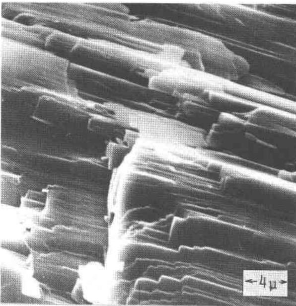
FIG. 2. Scanning electron micrographs of the fracture surfaces of jadeite. Note the extensive transgranular cleavage characteristics of the crack propagation.
