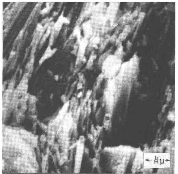
FIG. 3. Scanning electron micrographs of the fracture surfaces of nephrite. Note the fibrous nature of the fracture surface, the difference in fiber sizes, the occasional bundles of fibers, and the regions of random orientation.
