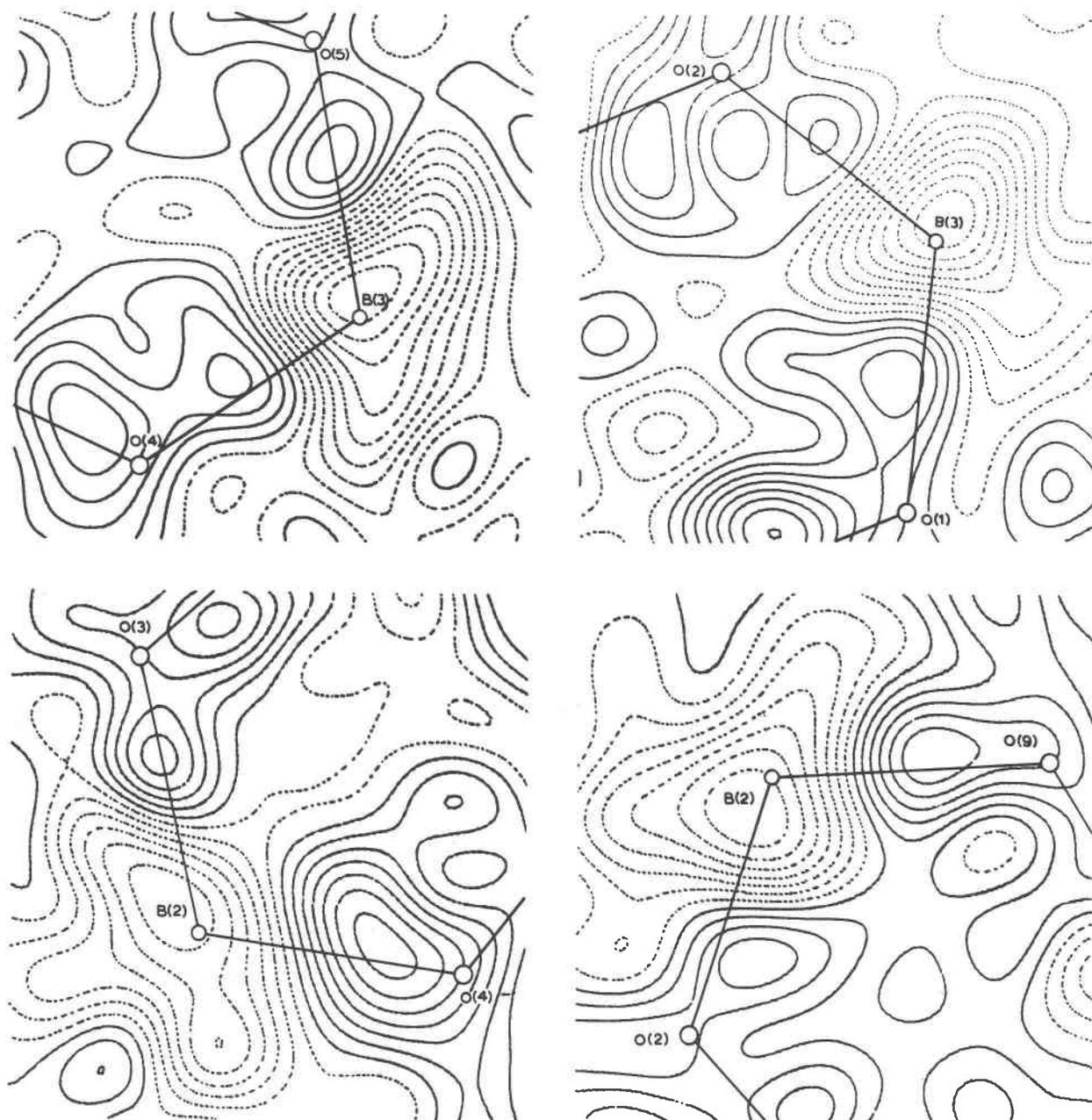
FIG. 4. Difference density maps. Contours at  $0.05 \text{ e}/\text{A}^3$ ; negative contours dotted. The sections shown lie in the plane of the boron and two oxygen atoms. The solid lines indicate bonds lying in the section.
