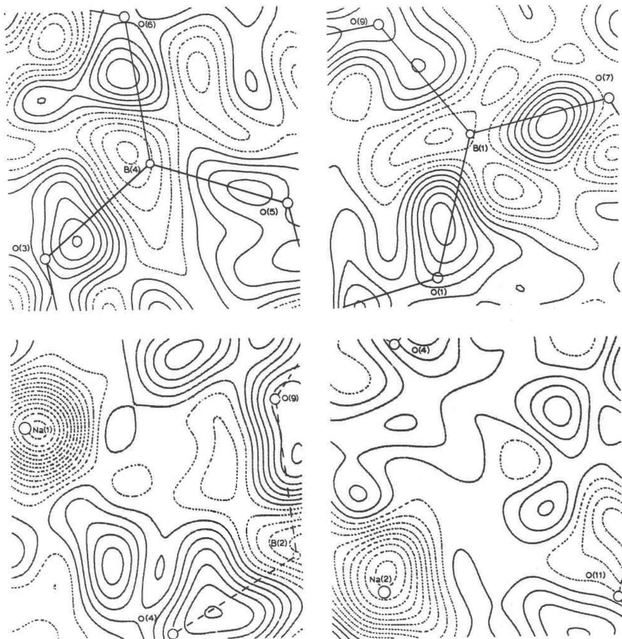
FIG. 5. Difference density maps. Contours at  $0.05 \text{ e}/\text{A}^3$ ; negative contours dotted. The sections in the upper half of the figure contain the three oxygen atoms, while those in the lower half are through one sodium and two oxygen atoms. The solid lines indicate bonds lying in the section; the dashed lines are projections of bonds to atoms not lying in the plane of the density map.
