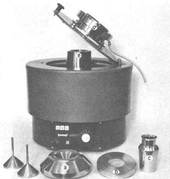
FIG. 2. The LOC separator. The letters of the components correspond to those in the diagram of Figure 1. Two accessory funnels (Fig. 3) are also shown.
