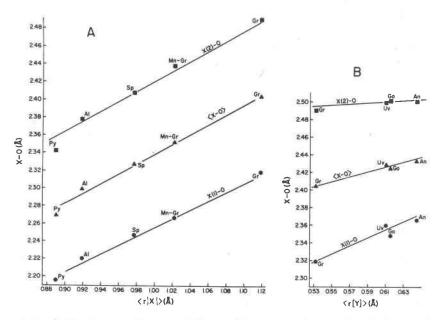
FIG. 7. Metal-oxygen distances, X(1)-O, X(2)-O, and their mean,  $\langle X$ -O $\rangle$ , of the triangular dodecahedron plotted against  $\langle r\{X\} \rangle$  for the Al garnets (A) and against  $\langle r[Y] \rangle$  for the Ca garnets (B).
