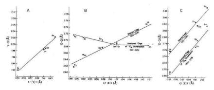
FIG. 6. Y-O bond distance plotted against  $\langle r[Y] \rangle$  for the Ca garnets (A). Shared octahedral edge, O(1)-O(4), and unshared octahedral edge, O(1)-O(5), plotted against  $\langle r[X] \rangle$  for the Al garnets (B) and against  $\langle r[Y] \rangle$  for the Ca garnets (C).
