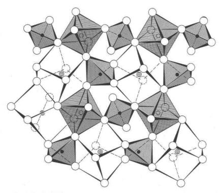
FIG. 1. Portion of the garnet structure projected down z showing the framework of alternating tetrahedra and octahedra (shaded portion) and the 8-fold triangular dodecahedra coordinating the  $\{X\}$  cations. The triangular dodecahedra are drawn as distorted cubes. Large open circles represent oxygens, smaller ones the [Y] cations, solid circles the (Si) cations, and the hatched ones the  $\{X\}$  cations.
