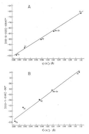
F1G. 5. Tetrahedral bond angle strain of the angle opposite the shared edge,  $[O(1)-Si-O(2)]-109.47^{\circ}$ , for the Al garnets plotted against  $\langle r\{X\}\rangle$  (A). Octahedral bond angle strain,  $[O(1)-Y-O(4)]-90.0^{\circ}$ , plotted against  $\langle r\{X\}\rangle$  for the Al garnets (B).
