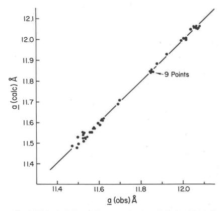
FIG. 2. Calculated cell edges a(calc) plotted against observed cell edges a(obs) for 56 silicate garnets, including 48 from other authors (Skinner, 1956; Abrahams and Geller, 1958; Geller and Miller, 1959c; Geller and Espenosa, unpublished data; Swanson *et al.*, 1960a; Swanson *et al.*, 1960b; Kohn and Eckart, 1962; McConnell, 1964; Geller *et al.*, 1964; Frondel and Ito, 1965; Strens, 1965; Prandl, 1966; Quareni and de Piere, 1966; Hsu, 1968; Huckenholz, 1969; and Moore *et al.*, 1969).
