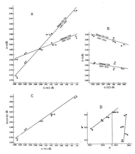
FIG. 8. Triangular dodecahedral shared edge length, O(4)-O(6), and unshared edge length, O(4)-O(7), plotted against  $\langle r\{X\}\rangle$  for the Al garnets (A) and against  $\langle r[Y]\rangle$  for the Ca garnets (B). Mean triangular dodecahedral edge length, TD $\langle O-O \rangle$ , plotted against  $\langle r\{X\}\rangle$  for the Al garnets (C). Tetrahedral-octahedral distortion parameter  $\beta$  plotted against the dodecahedral distortion parameter  $\phi$  (D).
