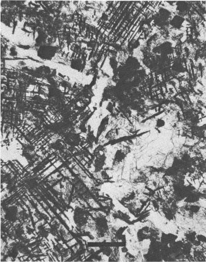
FIG. 1. Skeletal pseudobrookite, ulvospinel (irregular opaque grains), and pyrite (opaque cubes) in plexus of plagioclase, sphene, calcite, and chlorite. Bar scale equals 0.1 mm.
