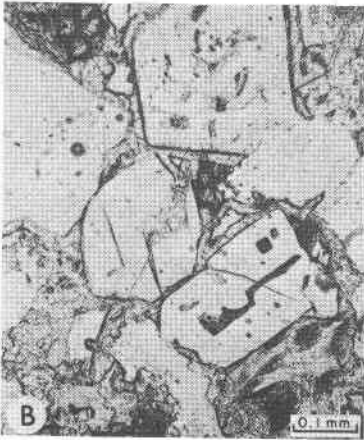
FIG. 3. Photomicrographs of tuff and tuffaceous sandstones from clinoptilolite zone. (A) clinoptilolite pseudomorph after glass shard, (B) clinoptilolite cement in tuffaceous sandstone, (C) close-up of clinoptilolite cement in tuffaceous sandstone.
