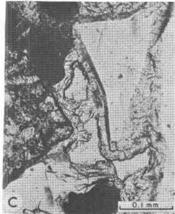
FIG. 3. Photomicrographs of tuff and tuffaceous sandstones from clinoptilolite zone. (A) clinoptilolite pseudomorph after glass shard, (B) clinoptilolite cement in tuffaceous sandstone, (C) close-up of clinoptilolite cement in tuffaceous sandstone.
