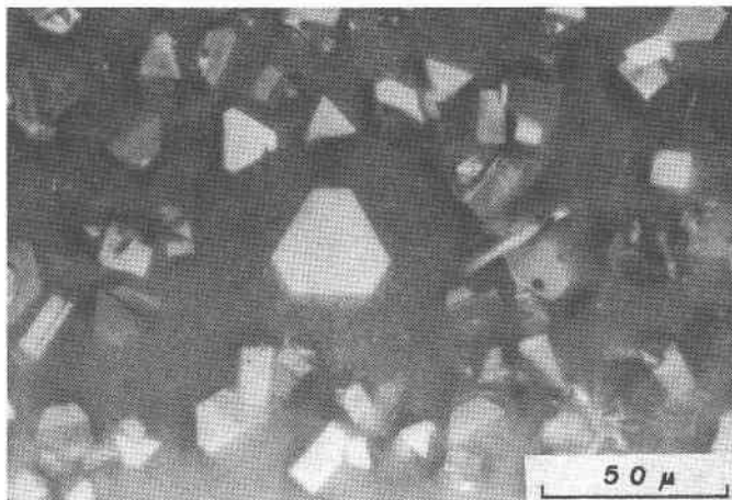
FIG. 2. Metastable cubic iron sulfide embraced in the ground-mass of the fine-grained mackinawite.
