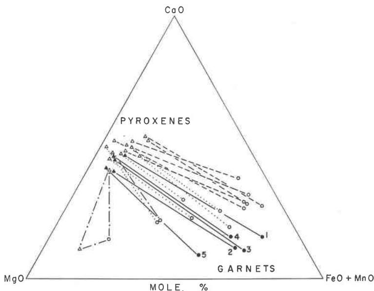
FIG. 6. C F M diagram for coexisting pairs of pyroxenes (triangles) and garnets (circles) in eclogites. Dashed-dotted tie lines: Group A eclogites; dotted tie lines: Group B eclogites; dashed tie lines: Group C eclogites. After Coleman *et al.* (1965, p. 504).
