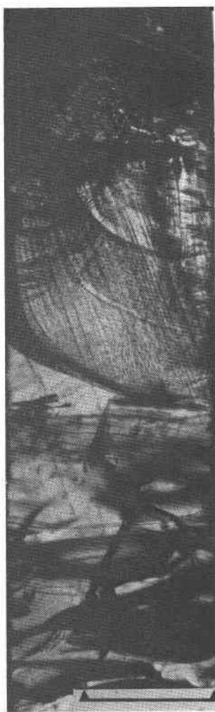
FIG. 8. Transmission optical micrograph of a specimen viewed between crossed polars and through (1\bar{1}00) , after 2% plastic compression in a direction 70^\circ from [0001] towards [\bar{1}120] . Strain rate 10^{-5} \text{ sec}^{-1} , temperature 800^\circ\text{C} . (Bar scale=1.0 mm).
