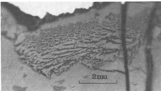
FIG. 3. Pseudographically intergrown ilmenite and iron-poor chromite with iron-rich chromite in the lower part of the picture. White is sulphide.
