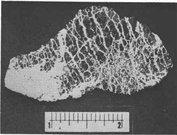
FIG. 7. Massive chromite showing pull-apart texture, Mine 133A, Jungtorghar. Scale in inches.
