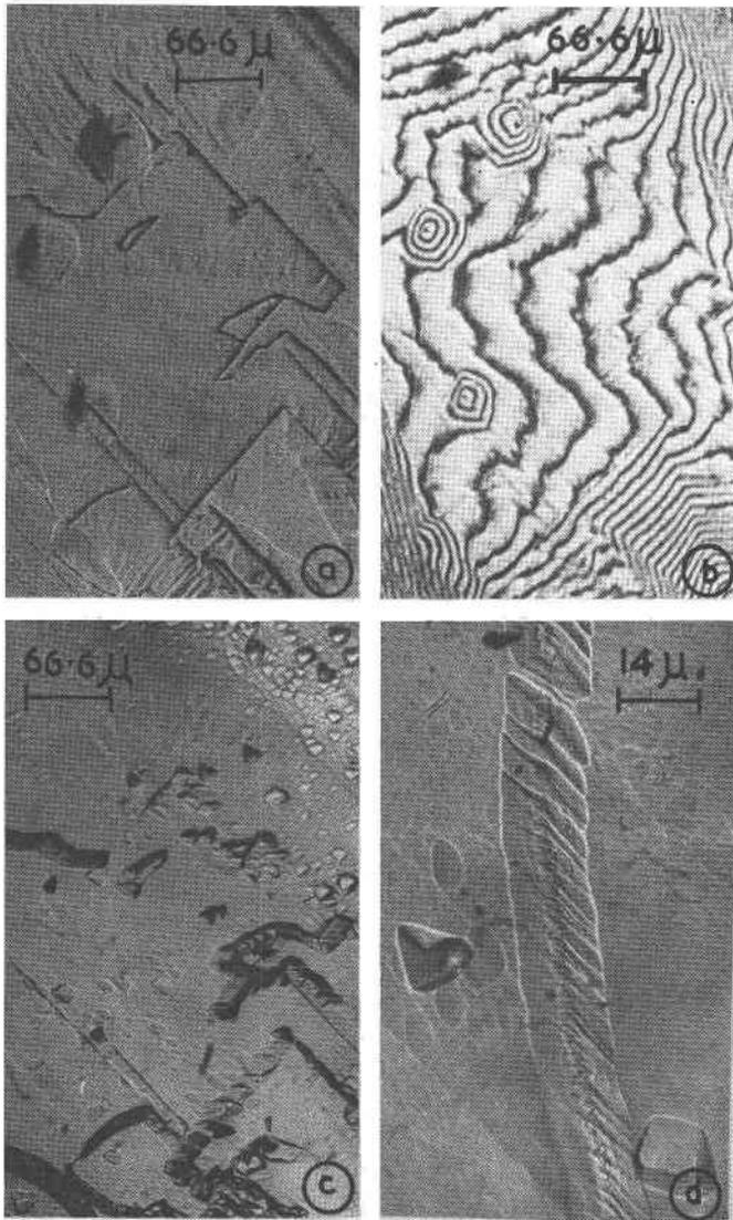
FIG. 13. Irregular boundaries: (a) Hillocks oriented at  $60^\circ$  within and outside an irregular boundary. (b) Interferogram over (a). (c) Etch pits oriented at  $60^\circ$  within and outside the boundary and replacing the corresponding hillocks of (a) Etchant KOH (d) Distorted etch pits on a portion of the line of discontinuity of (a).
