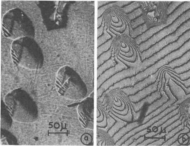
FIG. 8. Square hillocks slightly elongated to one side: (a) photomicrograph, (b) interferogram.
