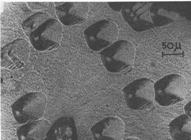
FIG. 7. Isolated hillocks with one side rounded.
