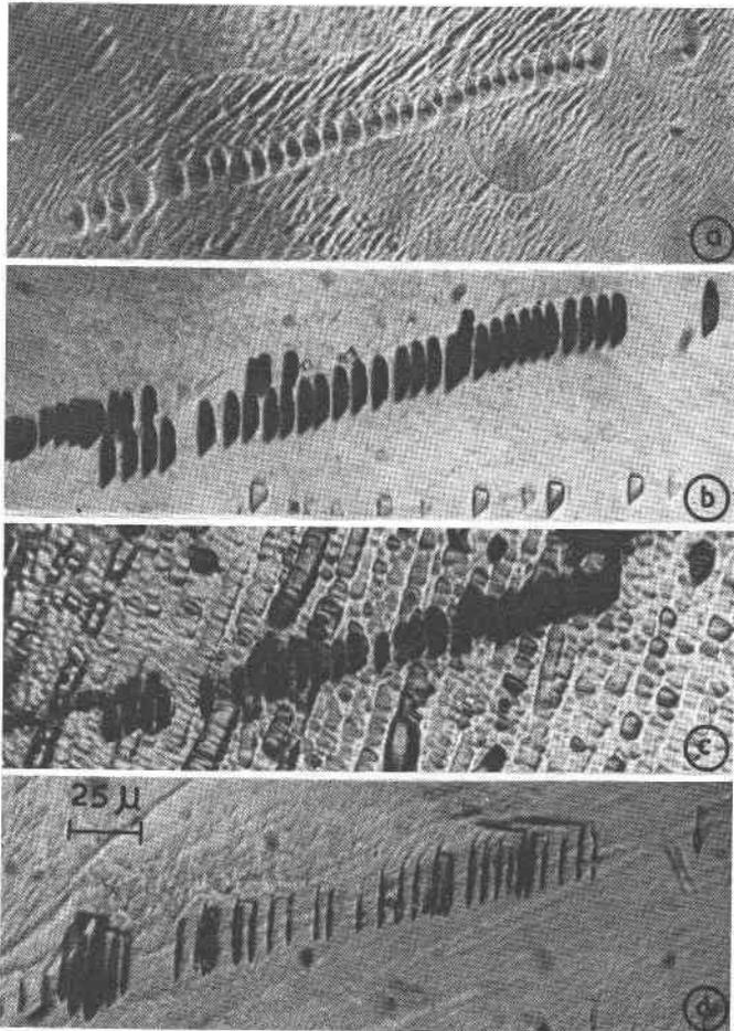
FIG. 5. An array of closely spaced square hillocks in (a); replaced in (b) by pits by etching in HF vapour; new pits in (c) produced after polishing and re-etching in KOH, showing exact correspondence with hillocks of (a) and pits of (b). In (d), pits produced after polishing and re-etching in HF vapour showing correspondence with hillocks of Fig. 5(a) and pits of Figs. 5(b) and 5(c).
