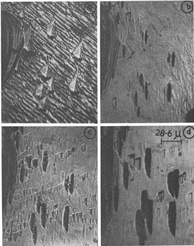
FIG. 4. Parachute-like hillocks. Hillocks in (a) etched into pits by HF acid vapour for (b) 30 (c) 50 and (d) 80 hours respectively.
