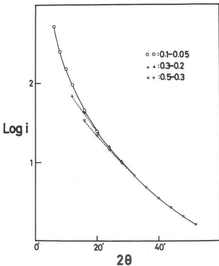
FIG. 3. A series of intensity curves for kaolinite. ○: slit system No. 1; Δ: slit system No. 3; □: slit system No. 4.
