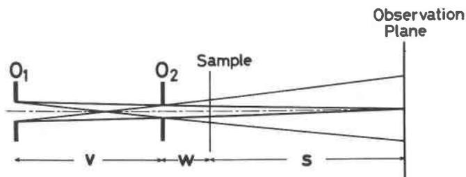
FIG. 2. Slit collimation system.  $O_1$ : 1st slit,  $O_2$ : 2nd slit.
