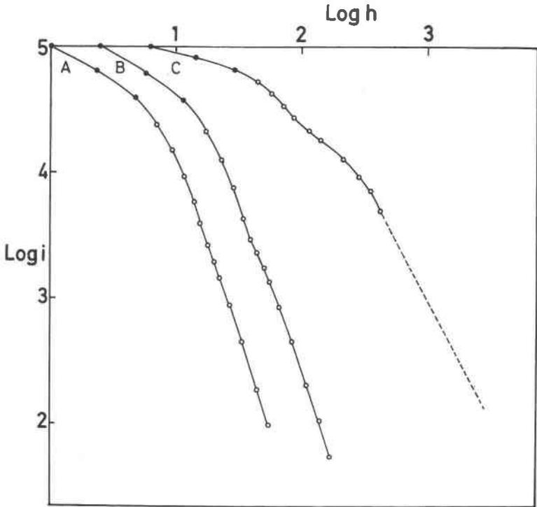
Fig. 5. The graph of  $\log i(h)$  versus  $\log h$  for clay minerals. A: kaolinite, B: hydrated halloysite, C: allophane. ○: observed; ●: extrapolated mathematically, broken line: extrapolated graphically.
