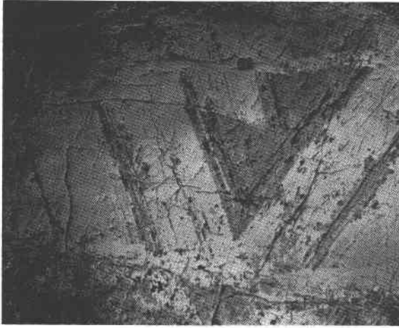
FIG 1(A). Zoned wolframite crystal from near Alice Springs, N.T., showing interzonal exsolution of scheelite, \times 13 .
