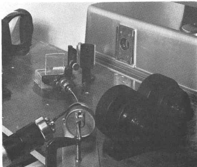
FIG. 2. Custom-made source unit for Model 12G Perkin-Elmer spectrometer. Sample, at focal point, is held in vertically-mounted mechanical microscope stage coupled to 12 RPH motor.
