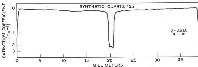
FIG. 7.  $\alpha_{3500}$  topograph for synthetic quartz crystal #125.
