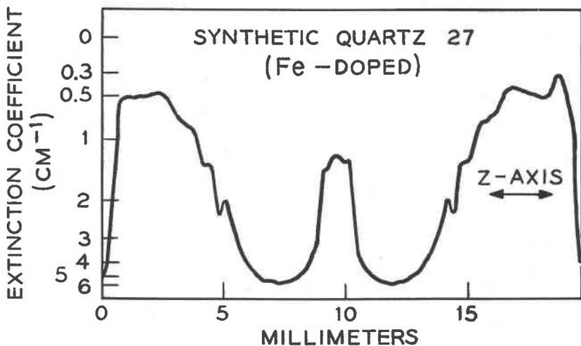
FIG. 5.  $\alpha_{3500}$  topograph for synthetic quartz crystal #27.
