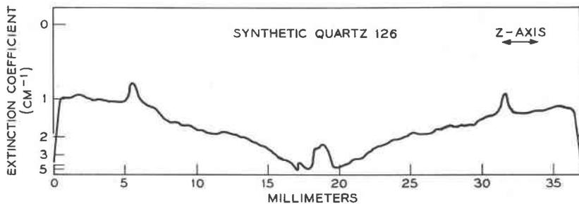
FIG. 6.  $\alpha_{3500}$  topograph for synthetic quartz crystal #126.
