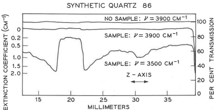
FIG. 3. Synthetic quartz crystal #86: Top trace: Scan at  $3900\text{ cm}^{-1}$  with no sample in beam. Middle trace: Scan at  $3900\text{ cm}^{-1}$  with sample in beam. Bottom trace: Scan at  $3500\text{ cm}^{-1}$  with sample in beam,  $\alpha_{3500}$  topograph.
