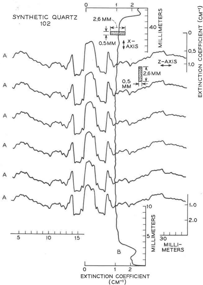
FIG. 4. Topographical  $\alpha_{3500}$  survey for synthetic quartz crystal #102.
