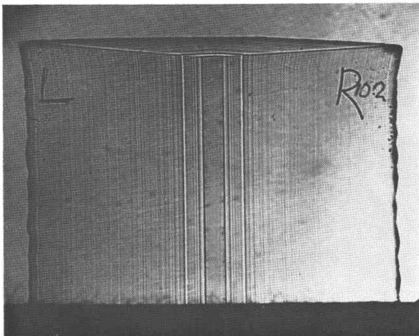
FIG. 1. Schlieren photograph of Synthetic quartz Crystal #102.
