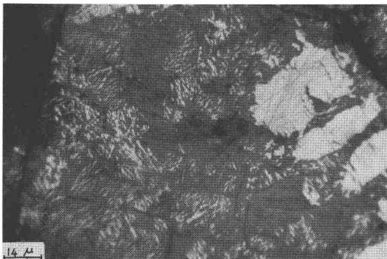
FIG. 3. Oriented network of very fine lamellae of mackinawite (white) in pentlandite. Incident light, oil immersion, nicols partially crossed.
