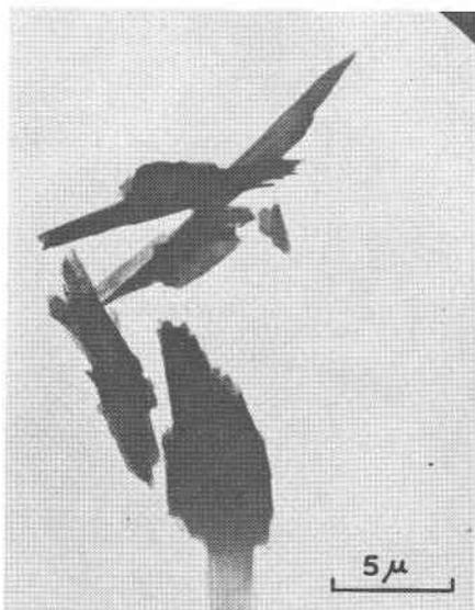
FIG. 5a. Electron micrograph of "abnormal" meta-jennite crystals.
