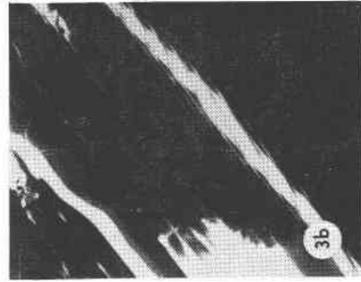
FIG. 1. Patterns of natural muscovite. (a) A type of dislocation lines. (b) A dislocation network.
