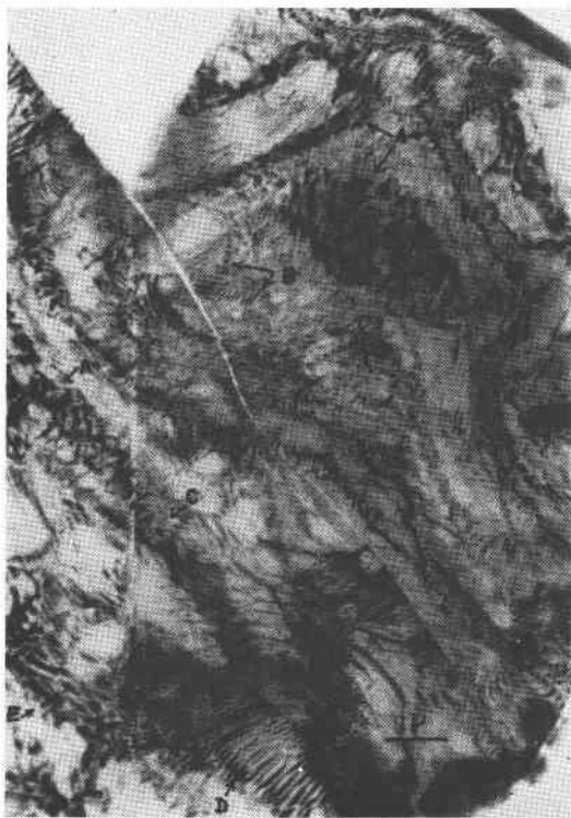
FIG. 4. A type of patterns of dehydroxylated phlogopite.
