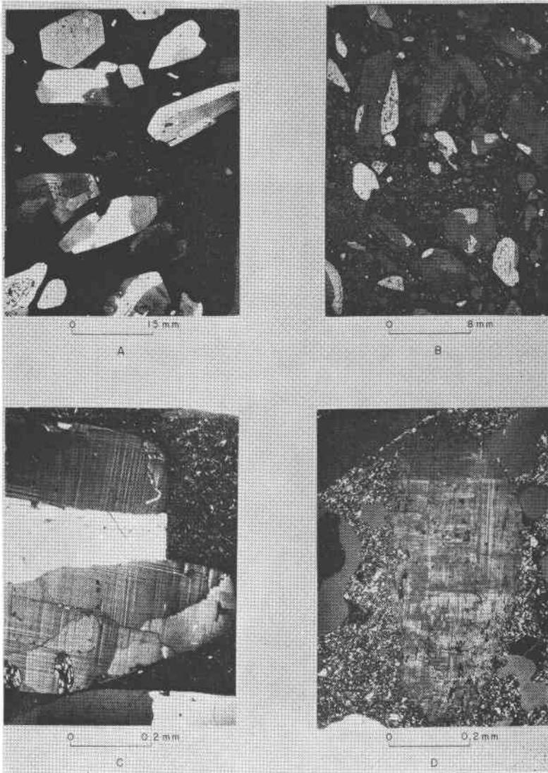
FIG. 2. Photomicrographs showing texture of anorthoclase trachyte BTB-8 (a) and FR-1 (b), and twinning in anorthoclase phenocrysts in BTB-8 (c), and FR-1 (d). crossed polars.
