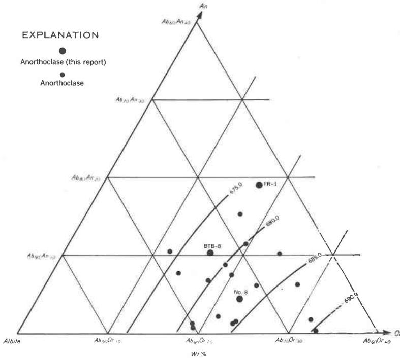
FIG. 6. Analyzed anorthoclase plotted in the Ab-rich corner of the ternary feldspar diagram showing variation in the cell volume (after Carmichael and MacKenzie; 1964, p. 955, Fig. 3). The comparison of anorthoclase of this report is shown (Table 5).
