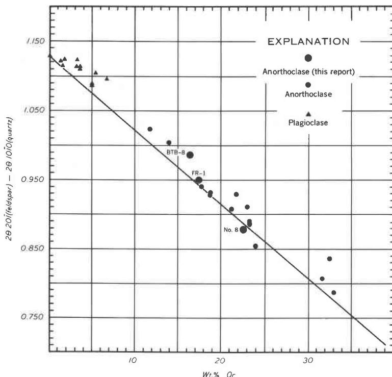
FIG. 4.  $2\theta(201) - 2\theta(10\bar{1}0)_{\text{quartz}}$  of anorthoclase and plagioclase plotted against Or content found by chemical analysis (after Carmichael and MacKenzie; 1964; p. 953, Fig. 1) showing comparison of anorthoclase of this report (Table 5).
