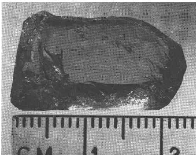
FIG. 5. ZnS crystal grown hydrothermally.
